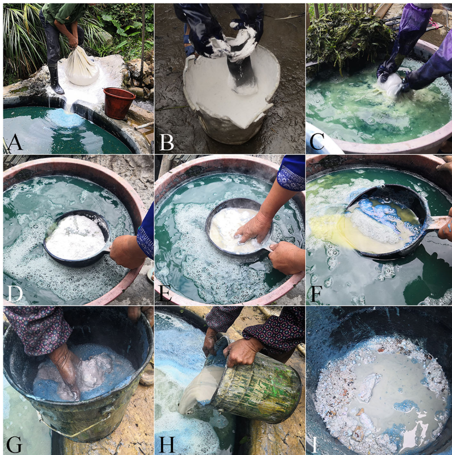
Fig. 7 The way in which lime is added in the process of indigo-paste production. a-c put lime into a cloth or gauze bag. d-i Put lime in a water scoop or bucket
