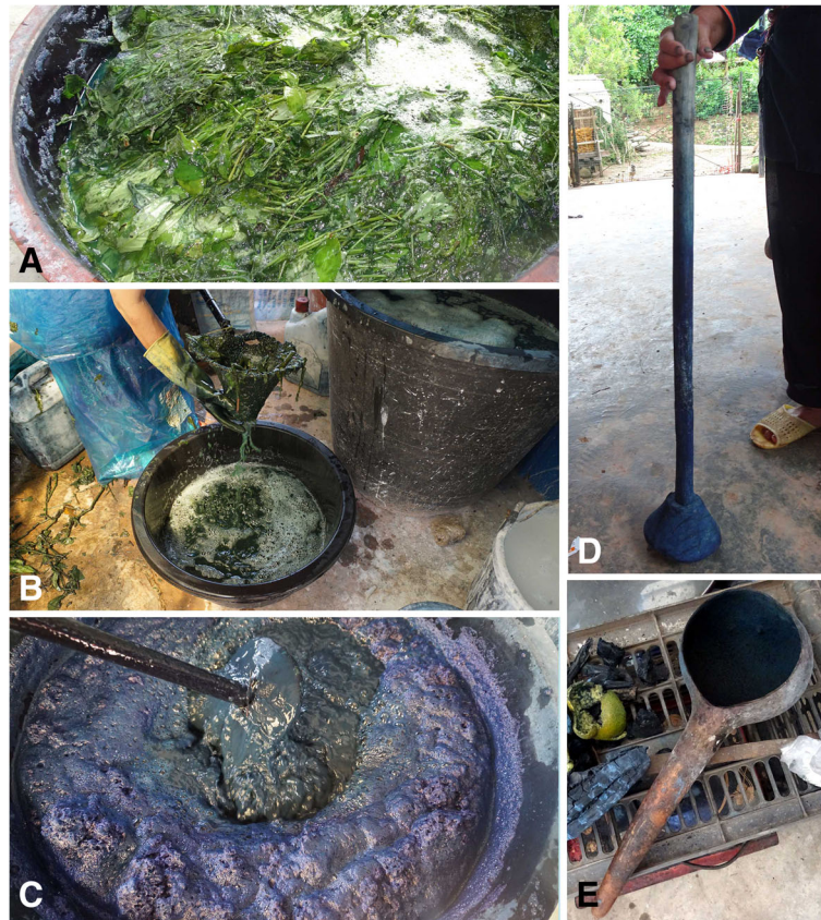
Fig. 4 The indigo paste production process. a Strobilanthes cusia leaves after 24 h of fermentation. b Removal of leaves using a net (called jiu in local name). c Oxygenation after adding lime water to reduce the pH. d Detail of wooden tool ( dongzhong ) used for oxygenation. e A half section of a gourd ( Lagenaria siceraria ) scoop used to take out indigo paste at the end of the process
